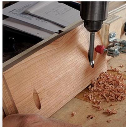
**Drilling at an angle.** The sharp rim makes it easy to start the bit in a steeply angled workpiece, as when cutting pocket holes in a table apron.
