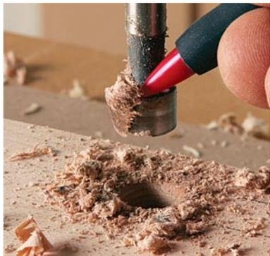
**Friction causes heat.** While cutting 100 holes in hickory, the temperature of each bit was recorded 10 times using a digital infrared thermometer. Bits that cut cleanly generated less heat.
