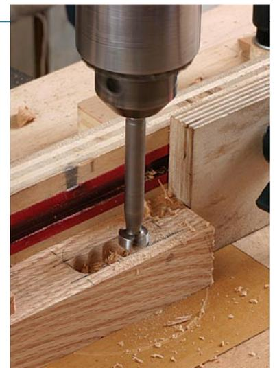
**Overlapping holes.** Again, the rim design allows you to drill clean overlapping holes, as when excavating a mortise.
